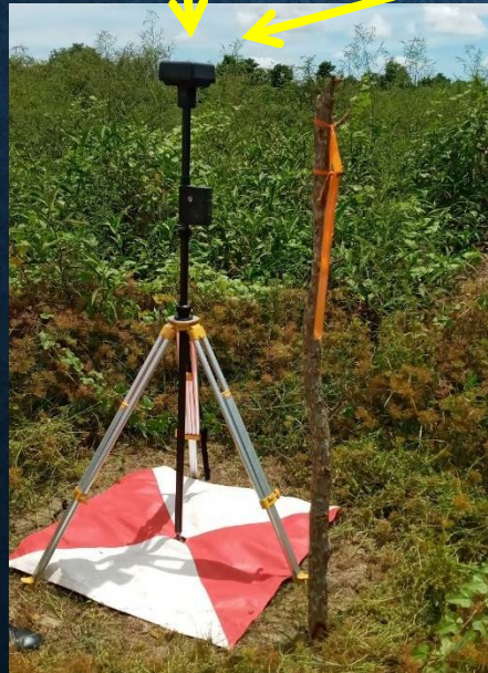
Mobile Base for RTK
