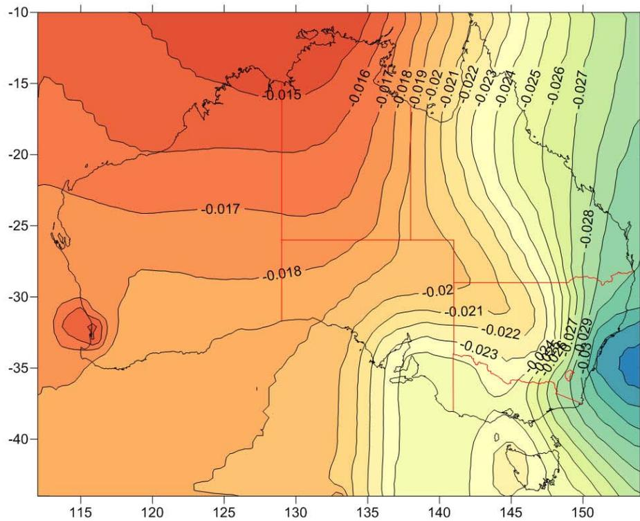
Figure 5. GDA94 to ITRF2008(1994.0) Coordinate Shift East (m)
