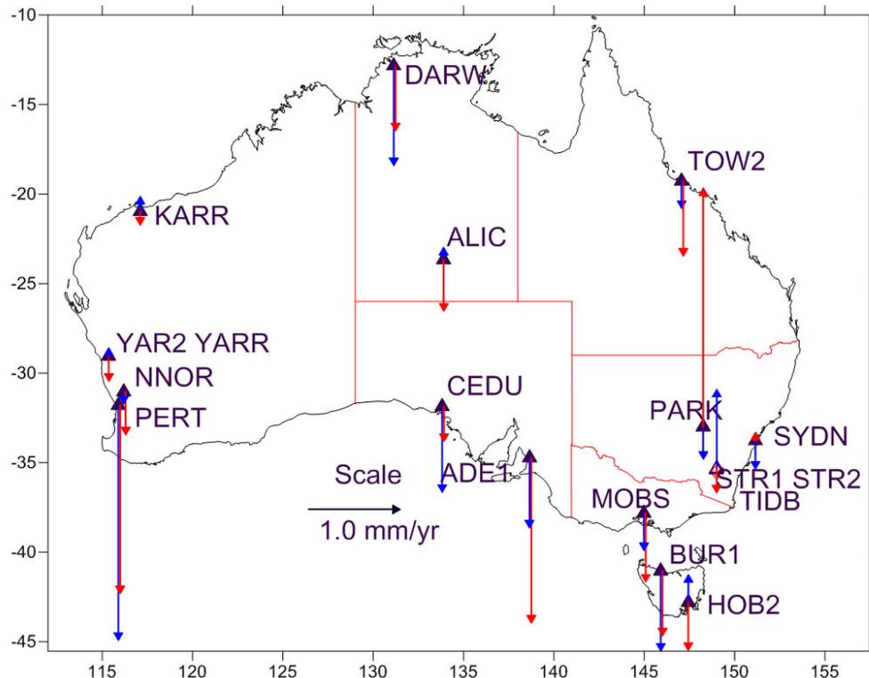
**Figure 2.** Observed vertical (UP) velocities at Australian fiducial CORS. The blue vectors show ITRF2008 GPS published vertical velocities. The red vectors show APREF observed vertical velocities.
