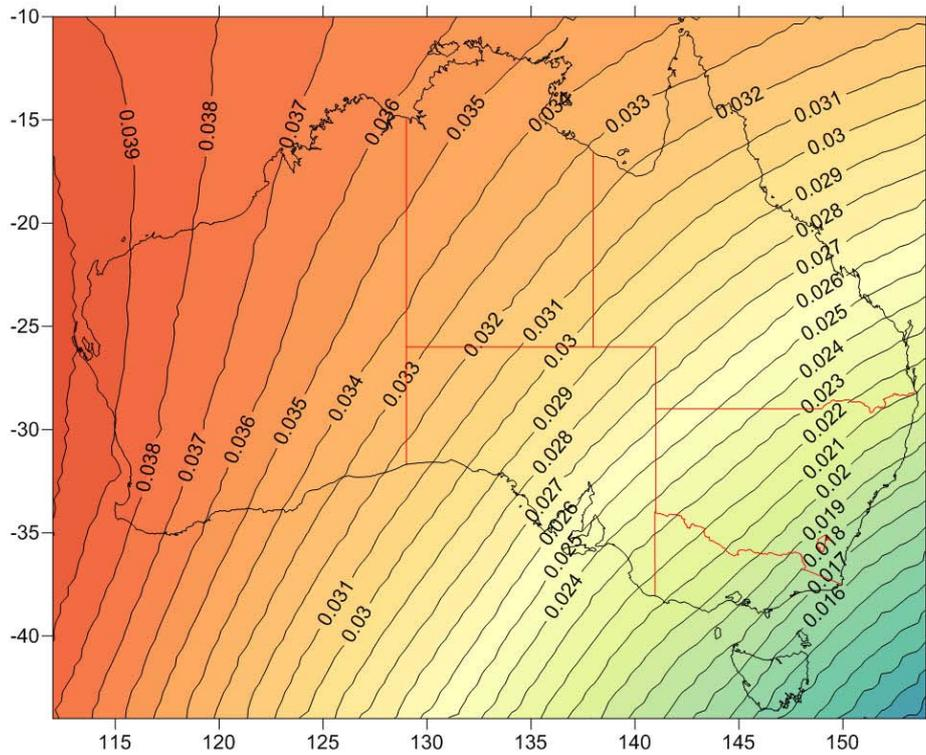
**Figure 3.** Australian Kinematic Model - Topocentric East velocity (m/yr)
