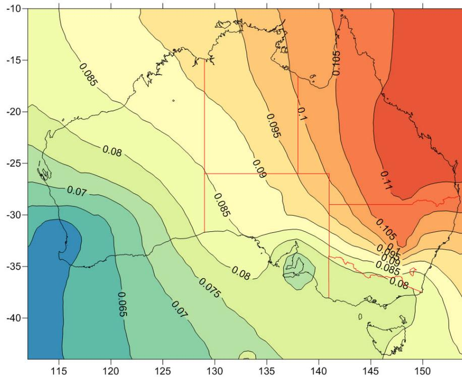
Figure 7. GDA94 to ITRF2008(1994.0) ellipsoid height correction (Up) (m)
