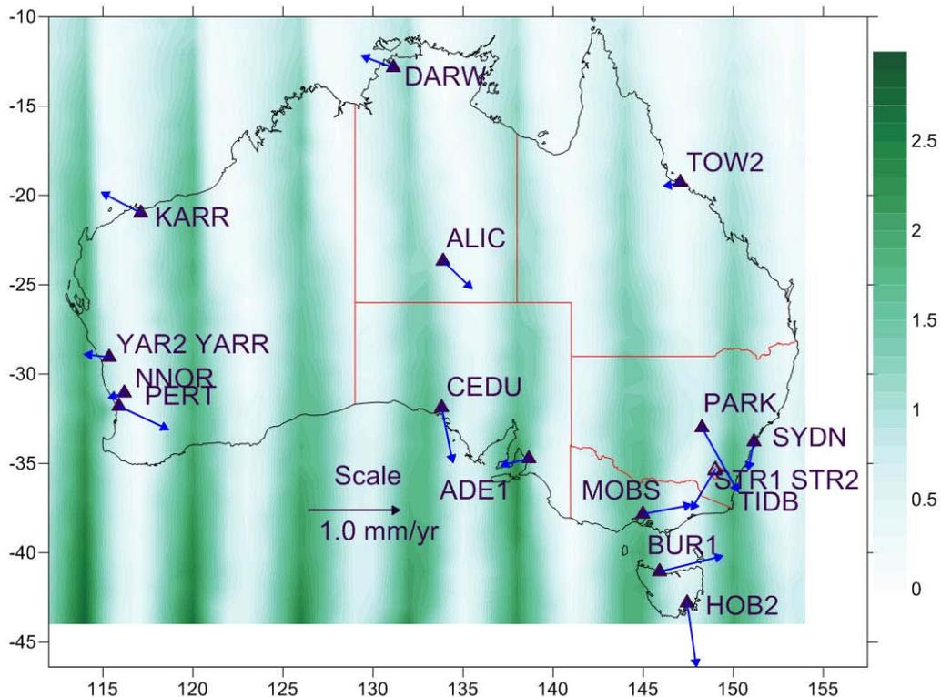
**Figure 8.** Comparison of Australian kinematic model with the current 14 parameter model (Dawson and Woods, 2010). Site velocity differences are shown by green shading (mm/yr). Blue vectors show APREF site velocities minus velocities estimated from the 14 parameter model.
