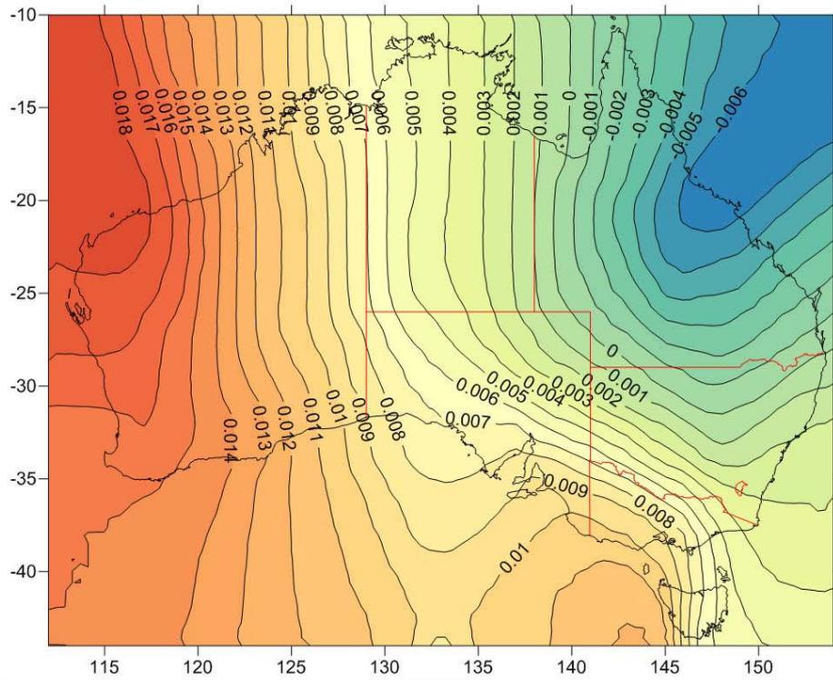
Figure 6. GDA94 to ITRF2008(1994.0) Coordinate Shift North (m)
