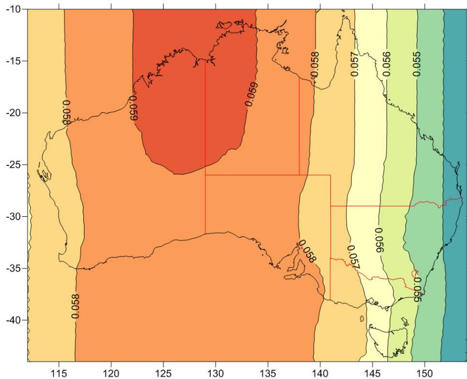
**Figure 4.** Australian Kinematic Model - Topocentric North velocity (m/yr)
