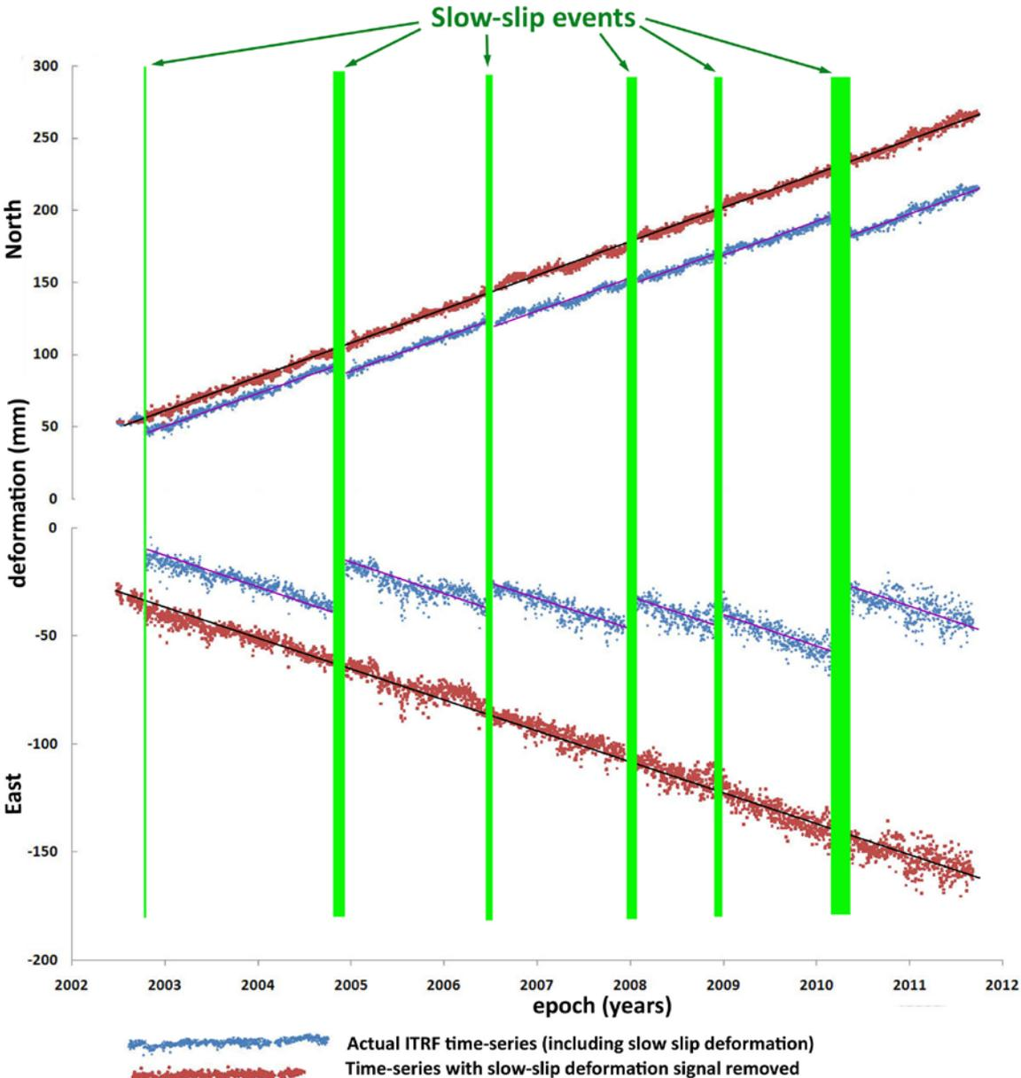
**Figure 9.** GPS time-series for GISB showing slow-slip events and trending interseismic velocities
