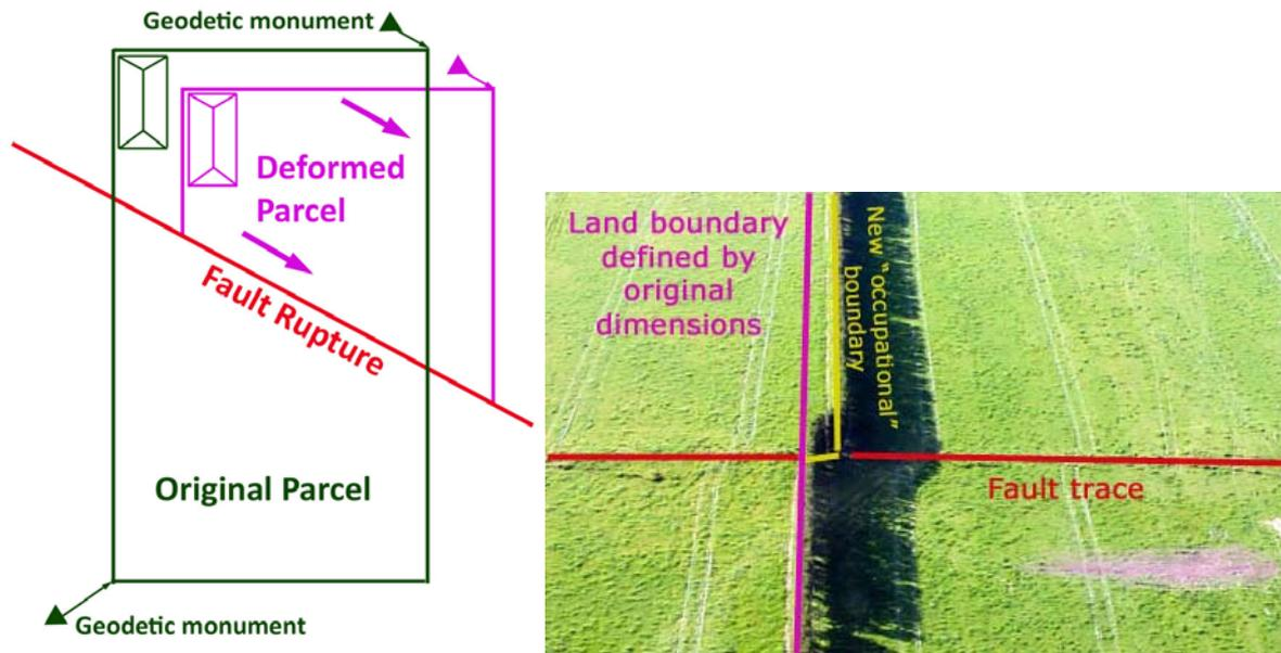
**Figure 2.** Effect of coseismic deformation on the cadastre and geodetic network.
