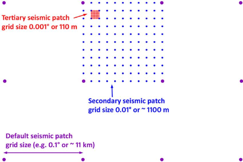
**Figure 5.** Nested structure of seismic patch grid model to accommodate localised deformation
