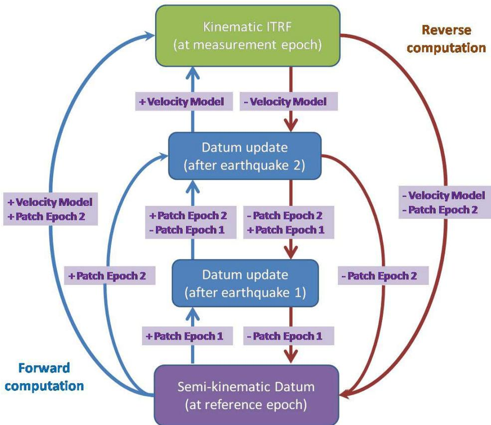
**Figure 4.** Flowchart showing transformation pathways between a semi-kinematic datum (fixed at the reference epoch) and kinematic ITRF.
