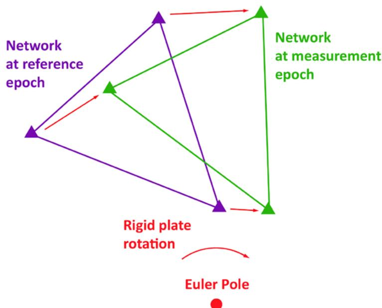
**Figure 1.** Schematic rigid plate rotation of network about Euler pole
