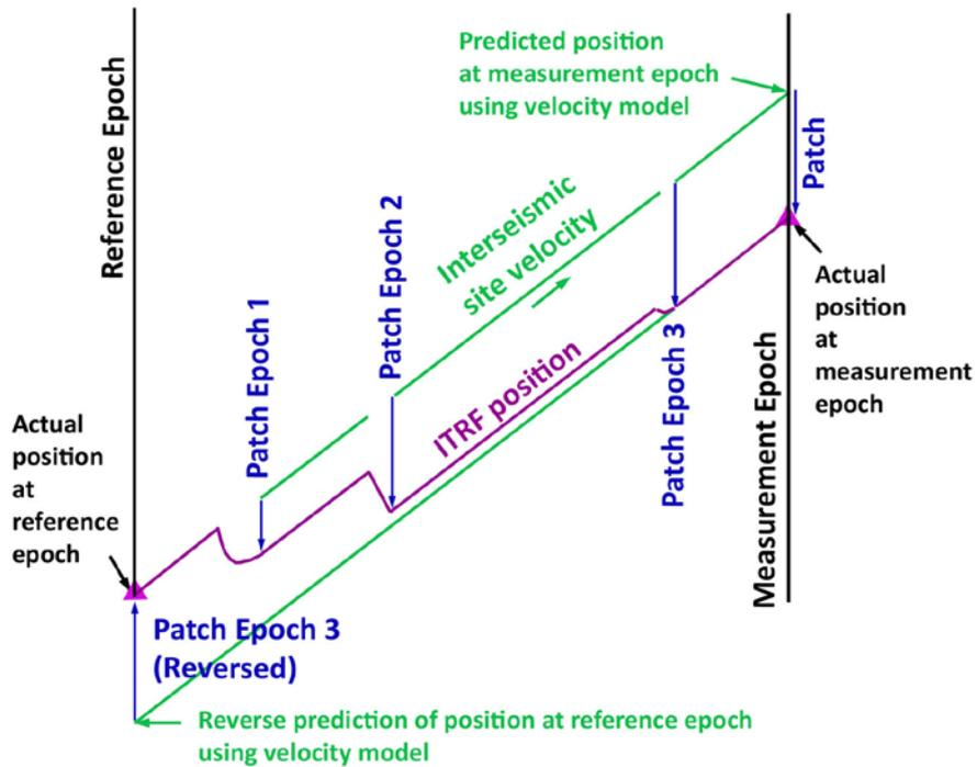
**Figure 3.** Schematic representation of the application of interseismic velocity models and seismic patches for deforming geodetic networks.
