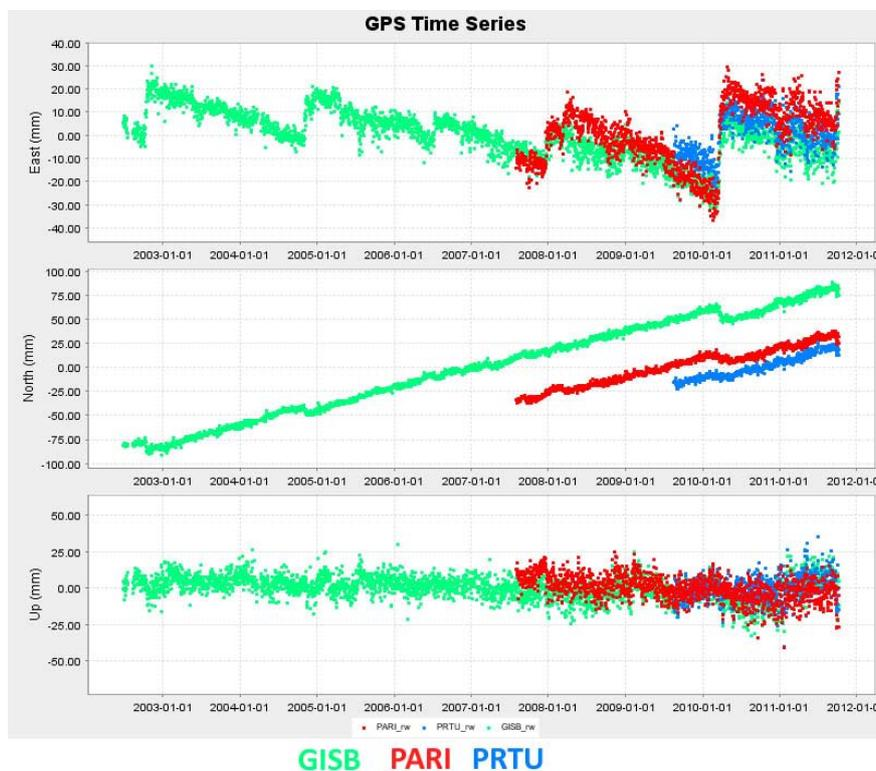
**Figure 8.** GPS time-series for CORS showing slow-slip events and trending interseismic velocities (GNS GeoNET web-site <http://www.geonet.org.nz/resources/gps/>)
