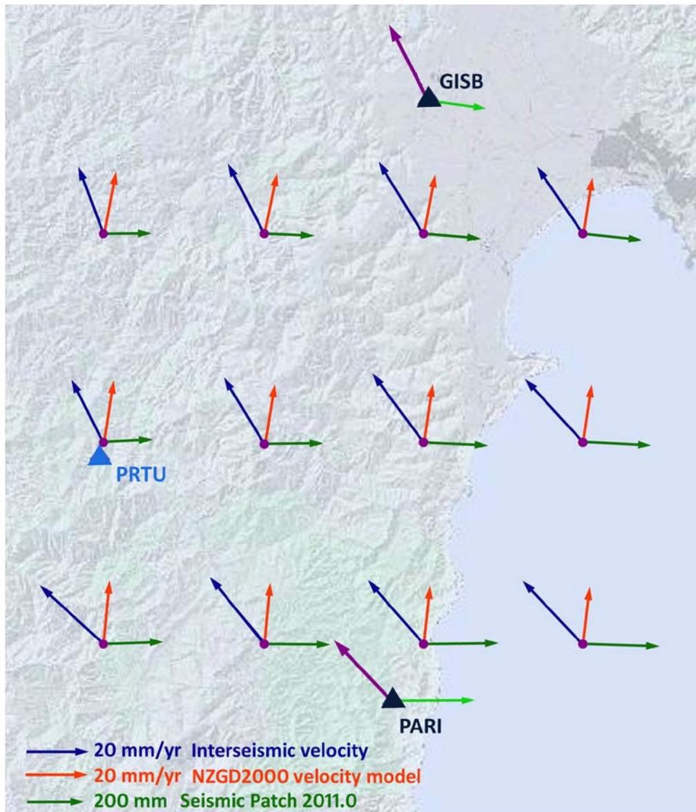
**Figure 10.** Deformation model for the case study area showing estimated interseismic deformation (blue), accumulated seismic deformation between 2000 and 2011 (green) and the New Zealand Deformation Model (NZDM) velocity estimates. Observed velocities and deformations at PARI and GISB are also shown.
