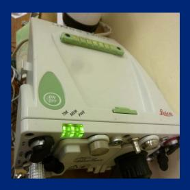
old Ashtech receiver and antenna replaced by Leica GRX1200 GNSS+ in October 2011. Using same antenna mount as MORE. 6 cm offset due to clay soil on site and tower damage. This required new site name.
