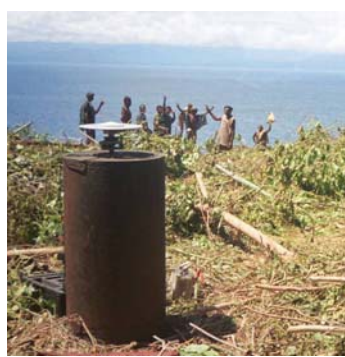
Figure 6 PNG Geodetic station on the Duke of York Islands used to monitor the Weitin Fault (visible in the background)
