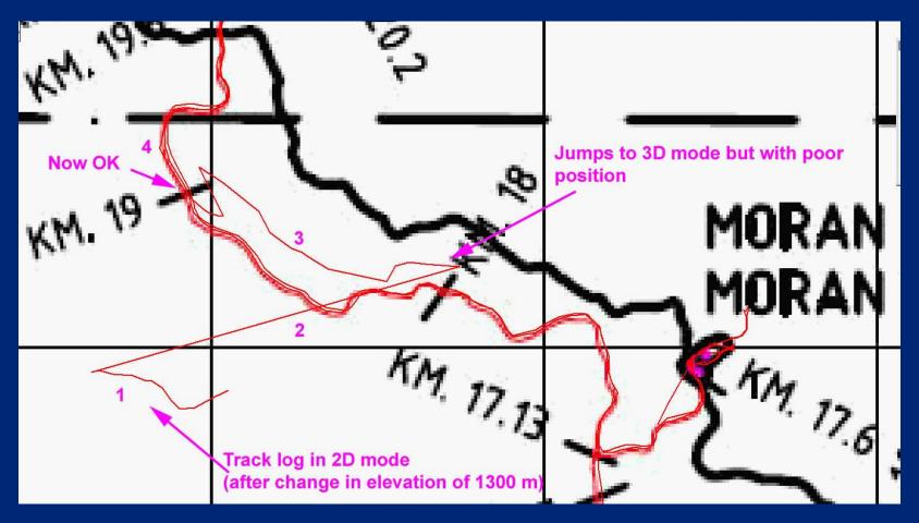
1.3 km position error in 2D due to change in elevation of 1300 metres!! This can be fatal.
